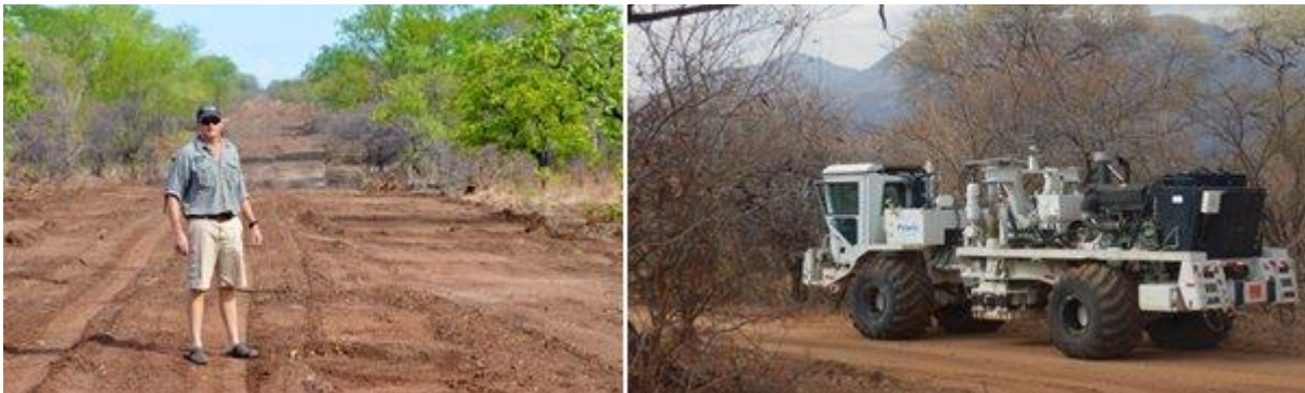
Figure 6. Example of swathe of track cut through mopane woodland to allow vibrator truck access for exploration purposes
